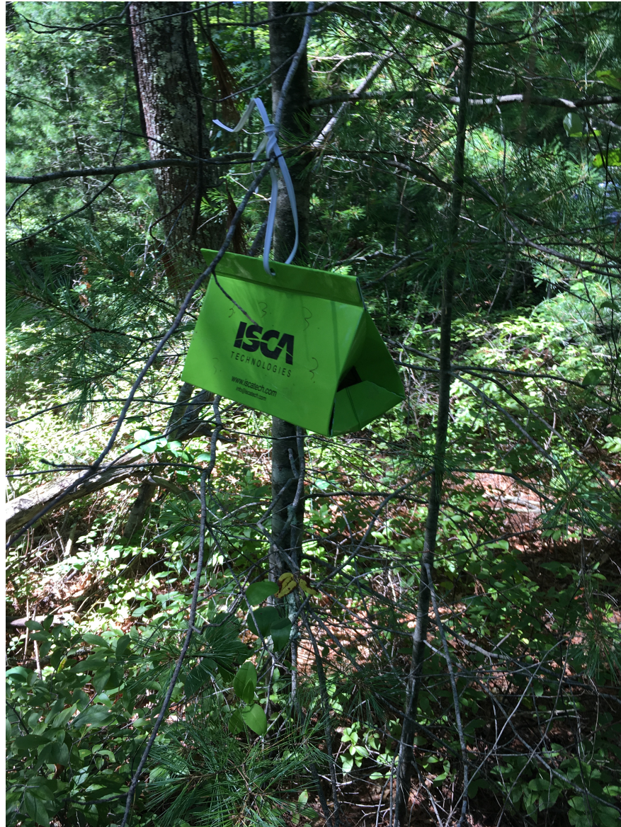
Figure A.12 Cardboard delta type trap used in Gypsy moth field trial.
