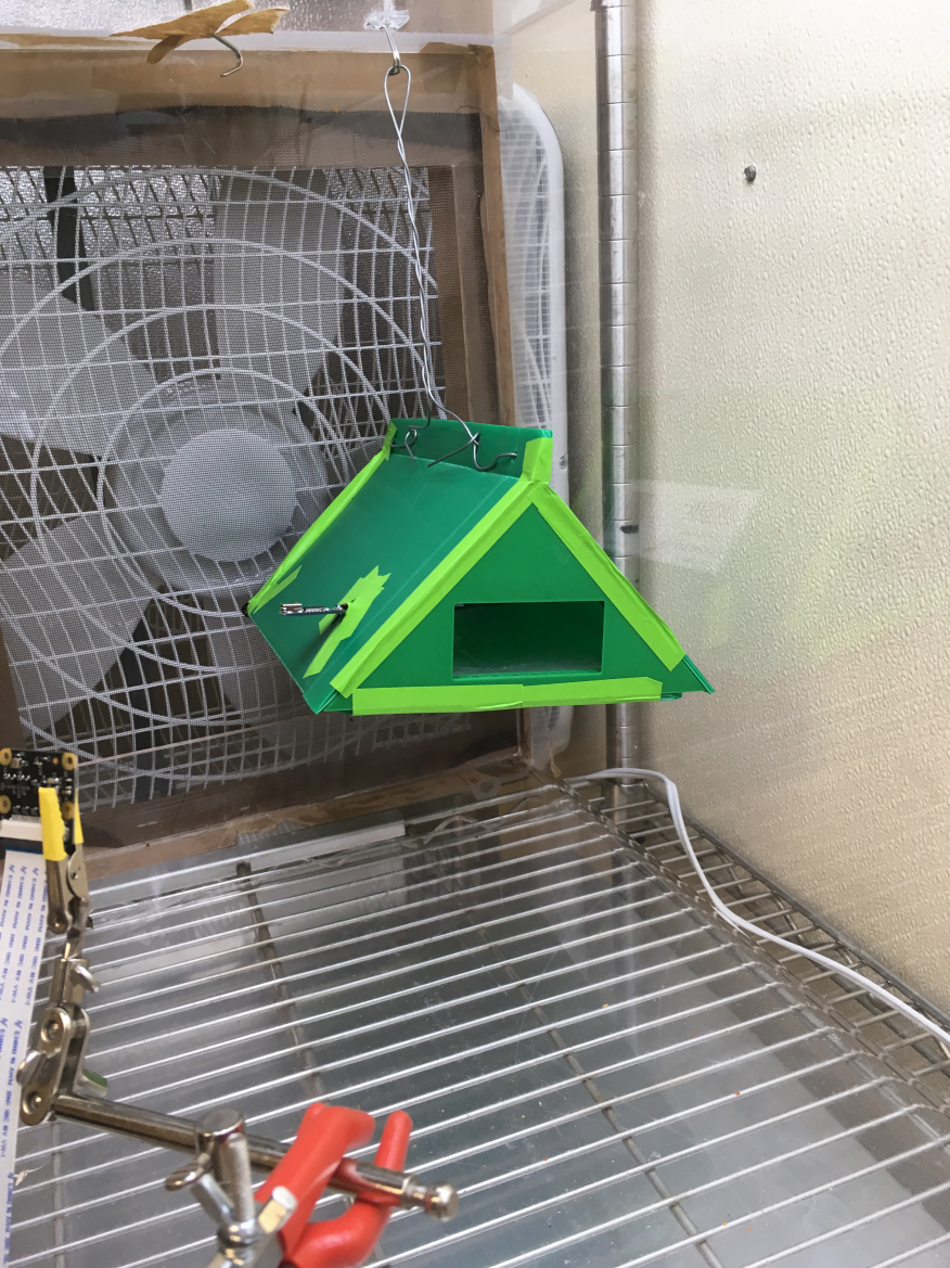
Figure A.11 Wind tunnel setup for Gypsy moth Experiment with sensor version 1.1.
