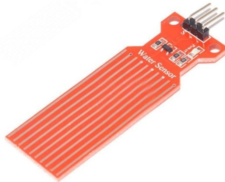
Figure 25. Resistive Water Level Sensor
