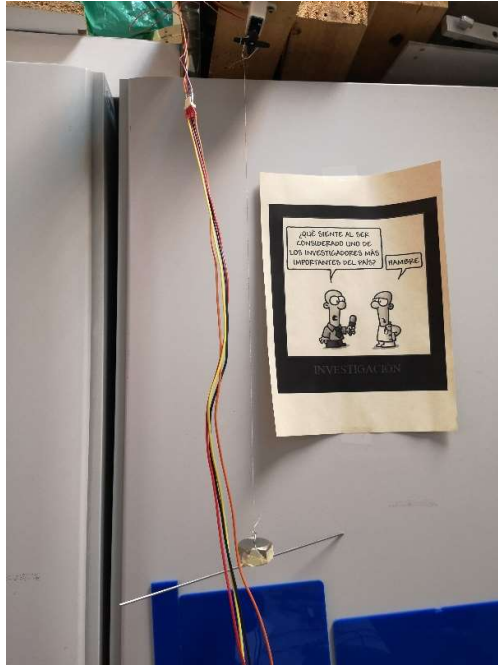
Fig. 3.5 The two loops of the thread are skewered onto the bent paperclip on the servo motor (top of the figure) and the hook on the weight.
