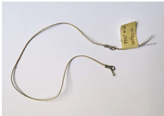
Fig. 4.11 The result of actuator 10 was more even than actuator 9 but the elasticity was not improved.
