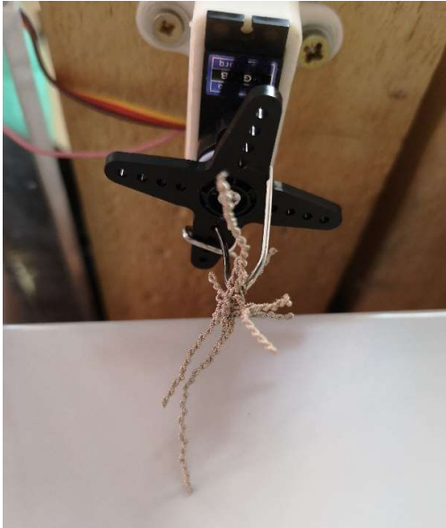
Fig. 4.12 When the thread broke it spun up towards the servo motor.
