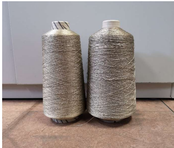
Fig. 3.1 The two different kinds of silver coated nylon yarn from Shieldex Trading Inc.. The left reel is Shieldex® 117/17 dtex 2-ply HCB and the right reel is Shieldex® 235/36 dtex 2-ply HCB.
