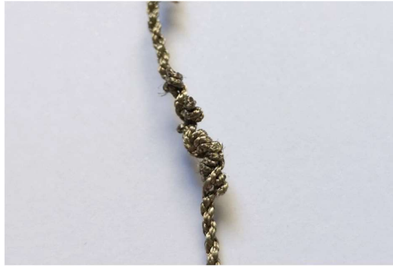
Fig. 4.10 A closer look at the groups of coils on actuator 9.
