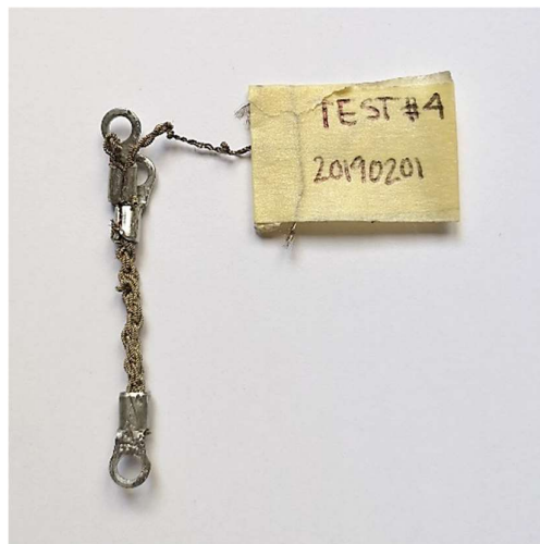
Fig. 4.5 The single thread 8 PLY actuator became very short and stiff.
