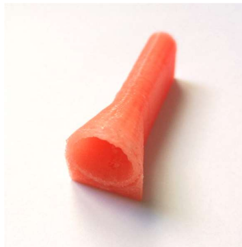
Fig. 4.48 First result of the manufactured guiding device for the rigidifiable material.
