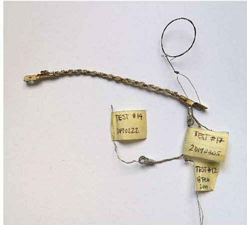
Fig. 4.15 Actuator 17 was a successful single thread 8PLY actuator made of two extended 4PLY actuators.
