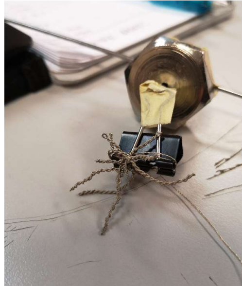
Fig. 4.13 The bottom part of the thread spun down towards the bulldog paperclip.
