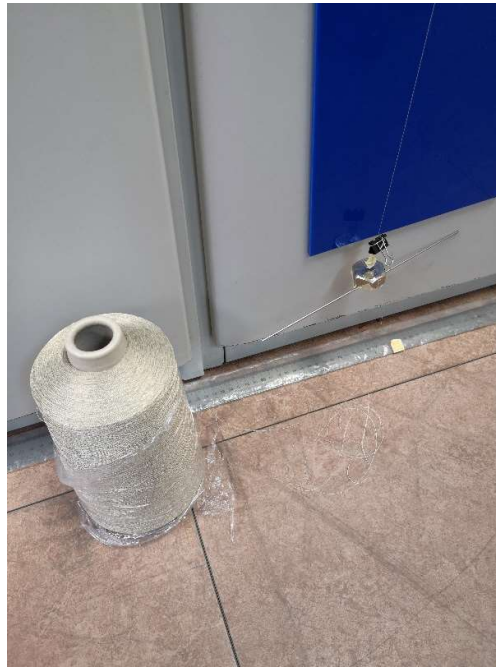
Fig. 3.7 The reel is placed on the floor besides the bulldog paperclip. A length of the yarn is lying loose on the floor.
