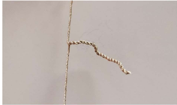
Fig. 4.6 Before the thread was fully coiled, coils grouped together and self-twisted.
