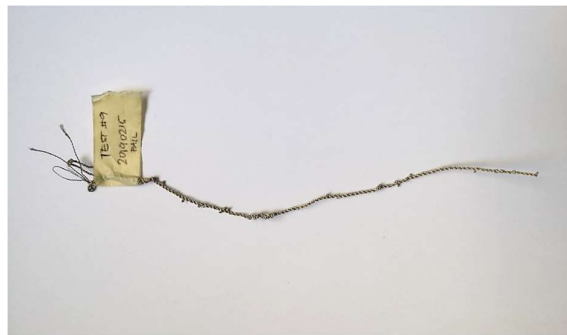
Fig. 4.9 Actuator 9 was uneven due to coils grouping together.
