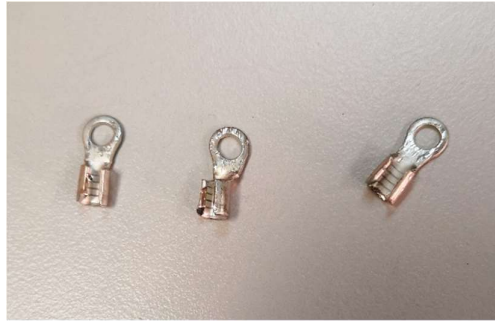
Fig. 3.12 Opened terminal ends used to crimp the ends of the manufactured actuators.
