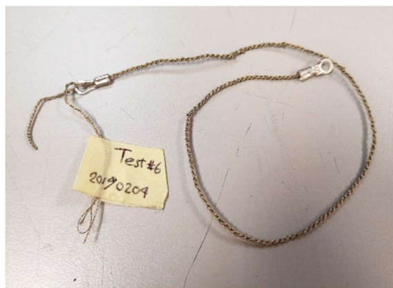
Fig. 4.7 Actuator 6 was tightly twisted and not very elastic.
