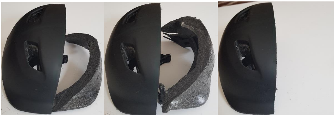
Figure 9: Cuts made to Helmet with Handsaw, 30^\circ Left Picture, 60^\circ Middle Picture, 90^\circ Right Picture.
