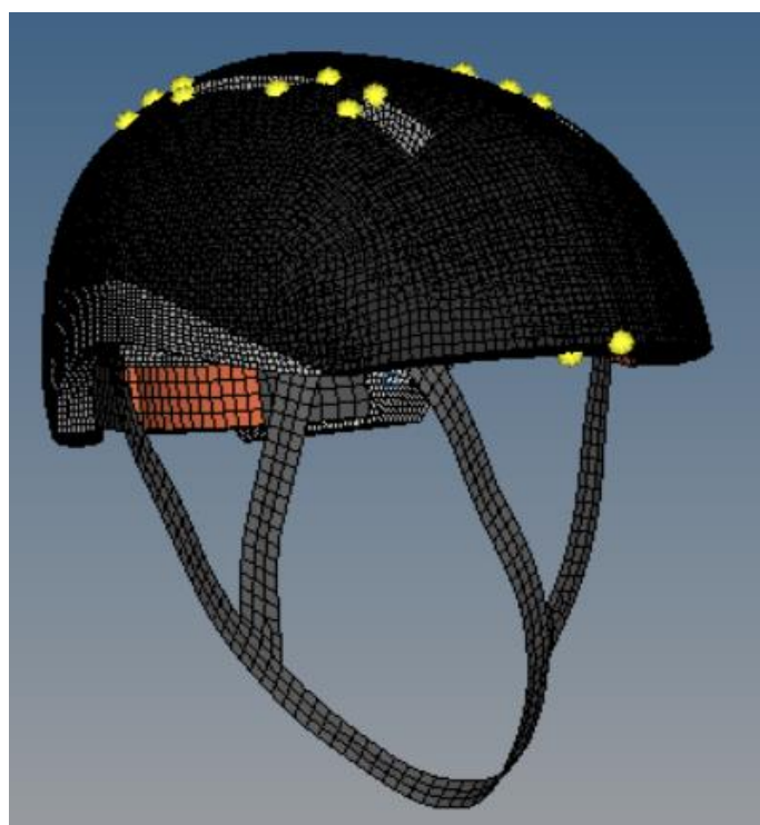
Figure 44: Mesh used for the Initial Simulation.
