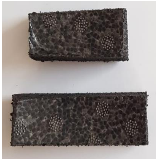
Figure 62: EPS Foam Samples from Helmet to Measure Density.
