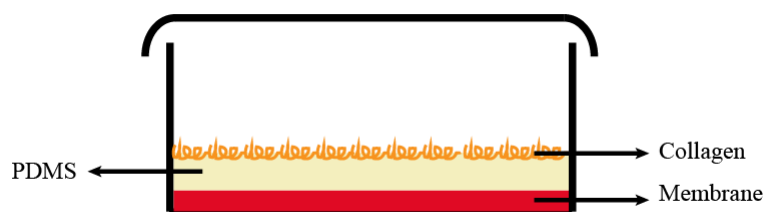
Fig. 3.2. Sensor assembled layers in a petri dish
