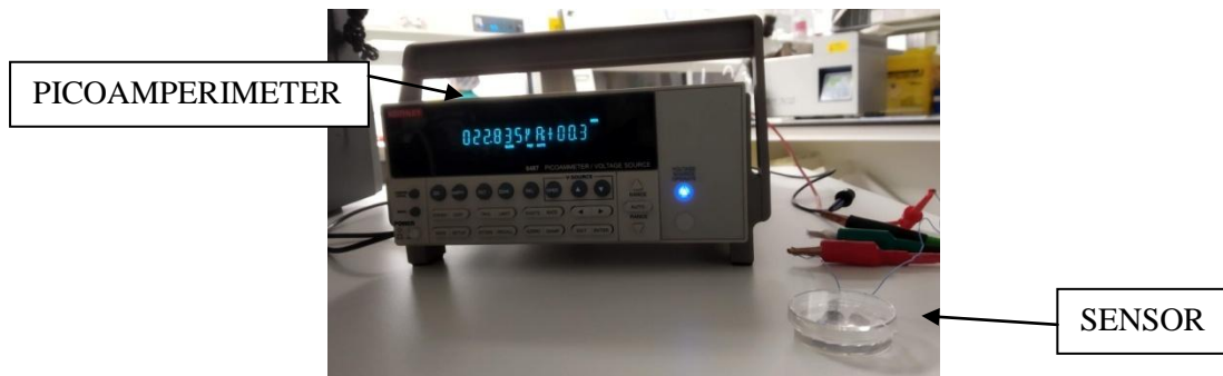
Figure 19. Picoamperimeter measurements assembly. The IDE was connected with the picoamperimeter by means of its copper cables.
