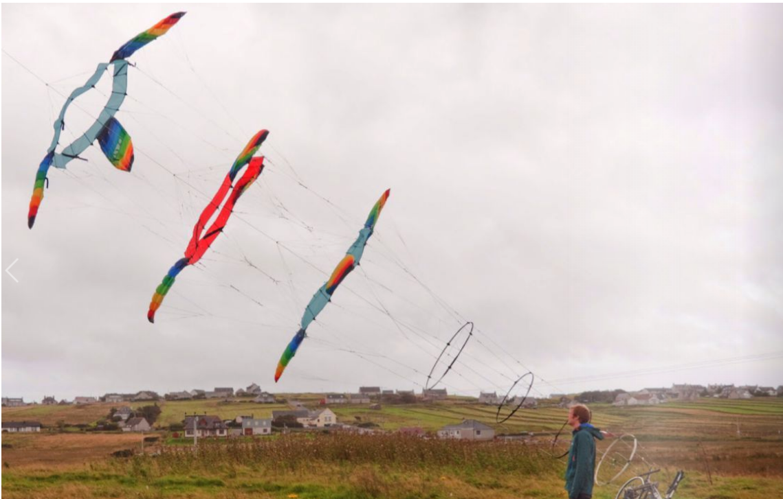
Figure 11: University of Strathclyde concept, rotatory system [4]
