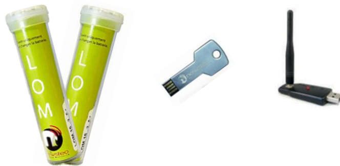
Fig. 8.1 Materials used: LOM16 RFID sensor, key containing the required software for visualization and receptor antenna
