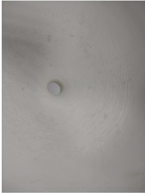
Figure 2.29: Close view of the interior of the nozzle. The wrinkled surface can be appreciated here, which remained even after the polishing with acetone.
