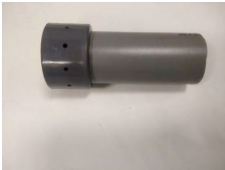
Figure 2.9: Machined lid of the impinging plate.
