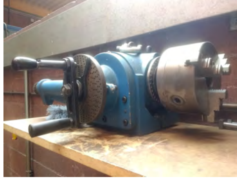
Figure 2.12: Angle variator that goes attached to the miller.
