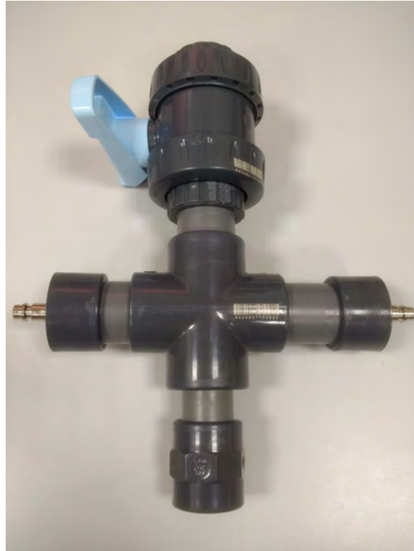
Figure 2.3: Mixing chamber. The light grey connections between the central cross and the ends are the glued PVC tubes.
