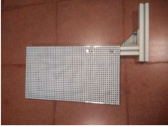
Figure 3.2: Calibration target for the camera.
