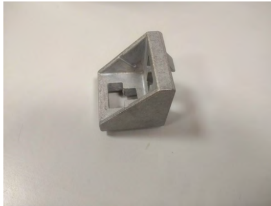
Figure 2.34: One of the brackets used for the profiles.
