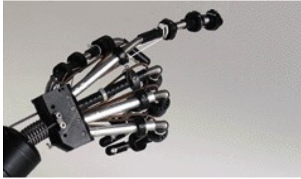
Figure 2.6: Robotic hand created with SMA. Retrieved from [6].
