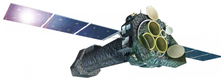
Figure 2.10: XMM-Newton satellite uses carbon composites for its main components [9]
