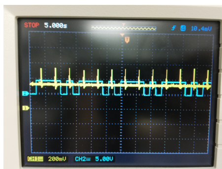
Fig. 5.5. TTL response when a simulated 20BPM signal is put into the gating device
