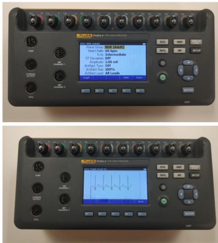
Fig. 3.8. Pro-sim 8 simulator options (above), and the graph of the signal generated (below).
