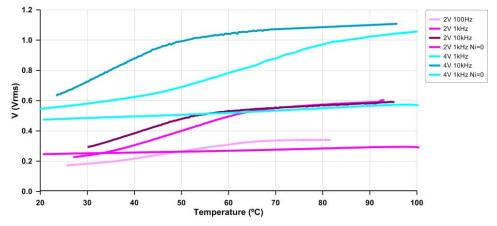
Figure 1. Frequency and voltage (rms) dependence of liquid crystal sensor response as temperature increases from 20°C to 100°C.
