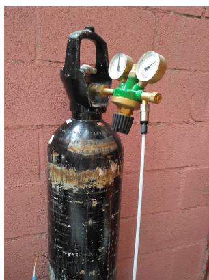
Figure 4.9. Purge gas cylinder
