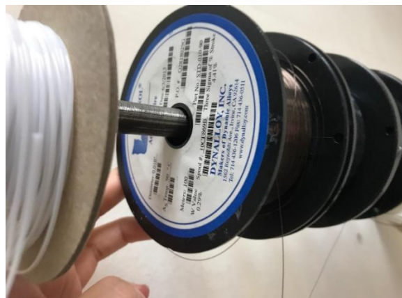
Figure 3.2.- SMA fibres - used for non-actuation purposes
