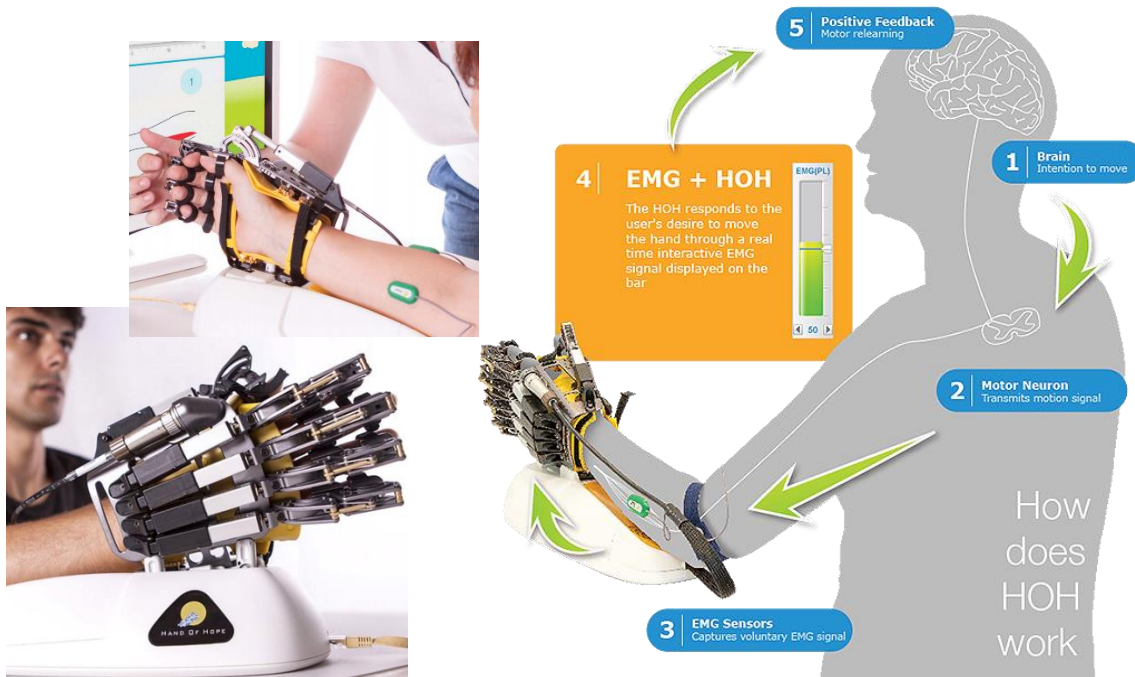
Figure 2.8.- Hand of hope and its working principle [29]
