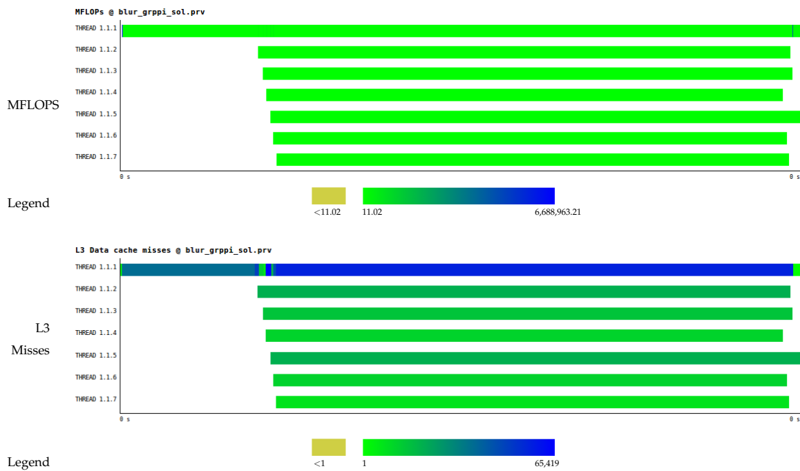
Figure 5-8: Trace of blur with Paraver tool. Top: MFLOPS metric. Bottom: L3 TCM.
