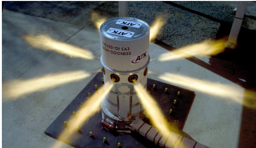
Figure 1: Attitude control system based on thrusters for a second Orion launch abort system developed by ATK being tested on ground.[1]
