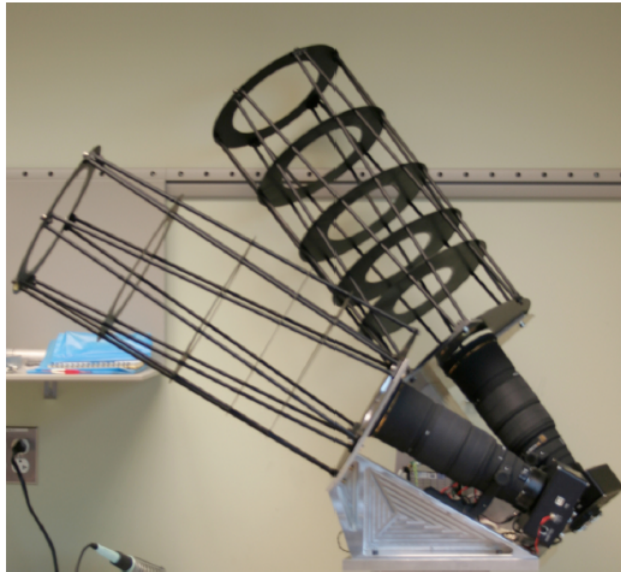
Figure 7: Star cameras used for the determination of attitude using the relative position of star in deep space. Baffles used to block light from lateral directions are missing leaving the cage exposed.[4]
