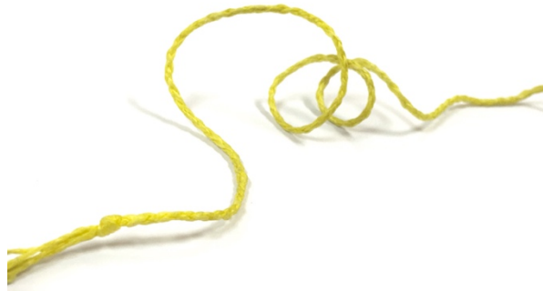
Figure 3.15 – Braid of Dyneema® Fishing Line
