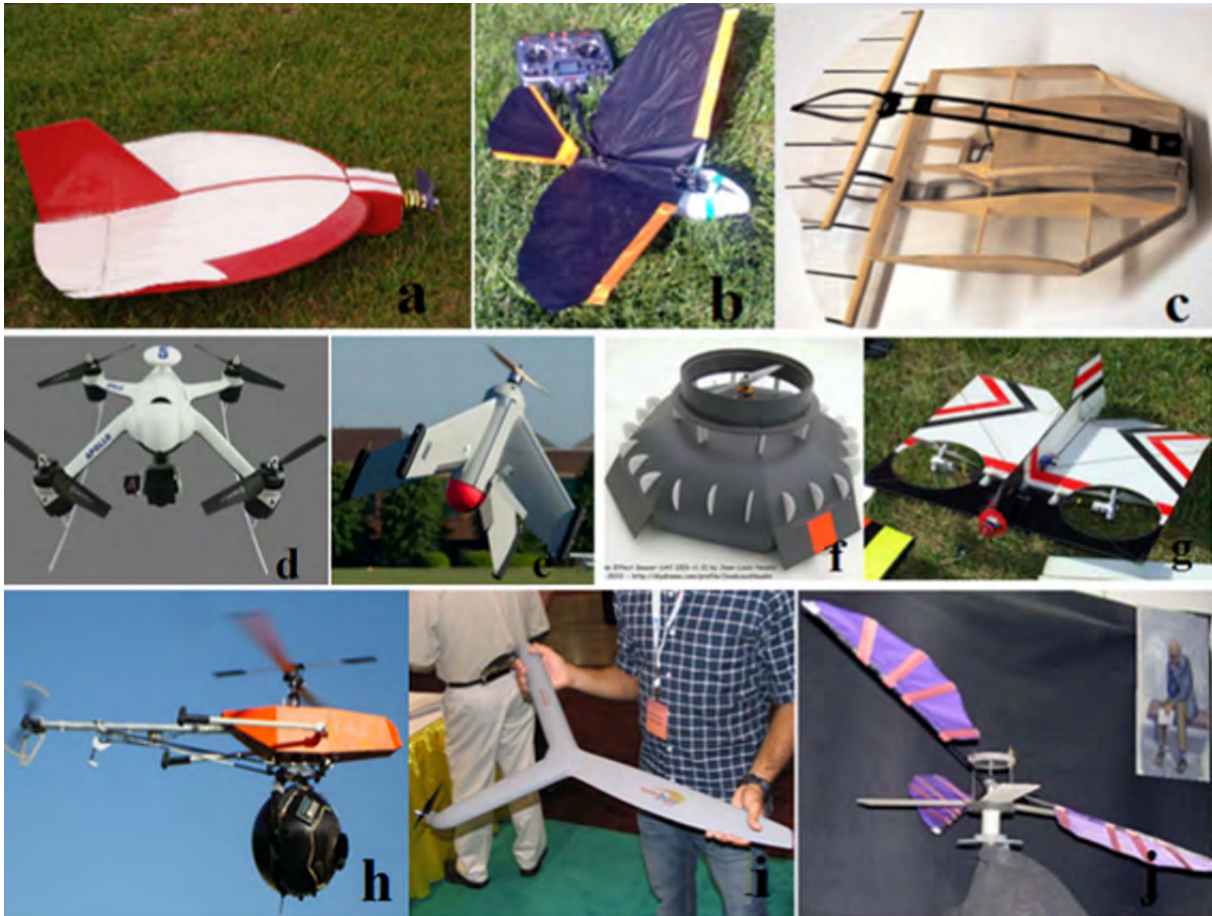
Figure 3: Classification of MAVs: (a) fixed wing, (b) flapping wing, (c) fixed/flapping-wing, (d) rotary wing , (e) VTOL, (f) ducted fan, (g) tilt-rotor, (h) helicopter, (i) unconventional, (j) ornicopter [8]
