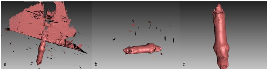
Fig. 5.3: Surface processing steps: a) Surface model without background removal. b) After background removal, small objects can be further cleaned. c) Final surface model exported.
