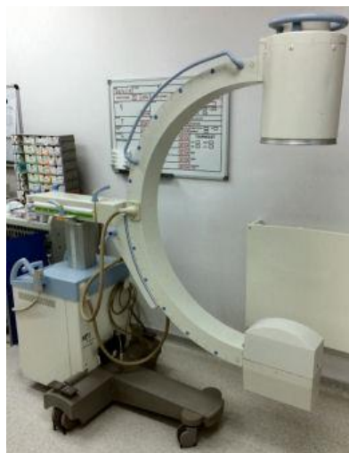
Fig. 1.12: A conventional C-arm system.
