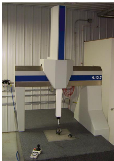
Fig. 3.1: A coordinate measuring machine (CMM) is shown as an example of contact based 3D scanner.
