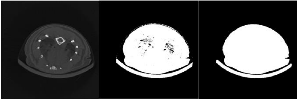
Fig. 5.2: Ideal reconstruction with FDK algorithm using a complete set of data (left), ideal mask obtained by thresholding (middle) and the final ideal mask after opening and hole filling (right).
