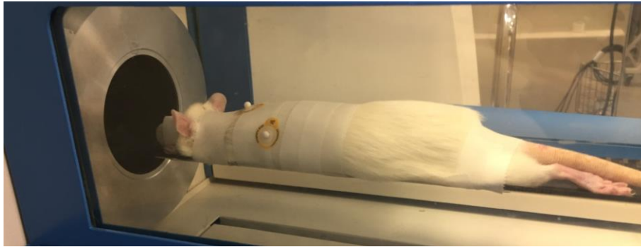
Fig. 4.2: Example of preparation of the sample with white tapes surrounding the thorax of the rodent and the bed to smooth the irregular hair texture of the sample
