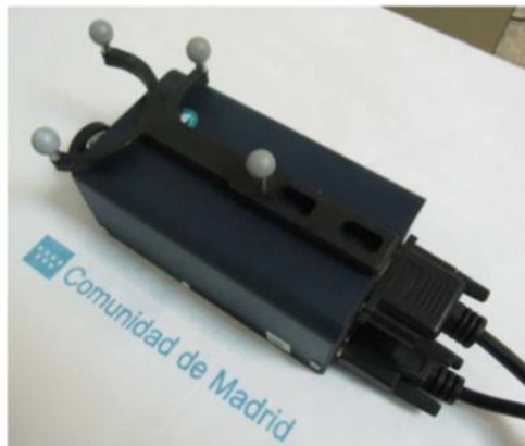
Fig. 3.4: Example of a conoscopic system: ConoProbe. Source: [21]
