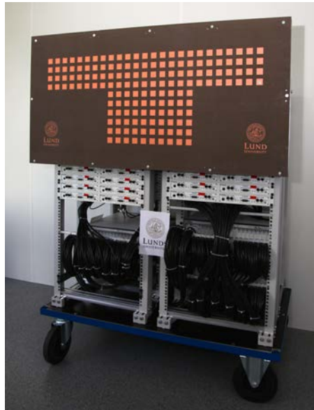
Figure 1.2: Prototype of massive MIMO equipped with 128 antennas at University of Lund.
