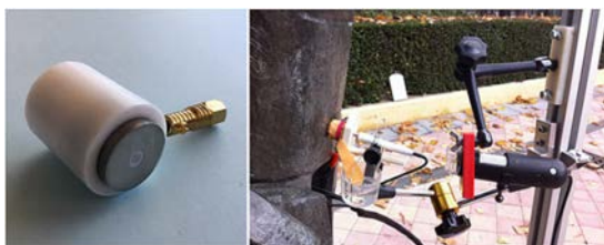
Figure 1. Contact probe designed by Paola Letardi. Cell construction (left) and complete measurement setup (right).
