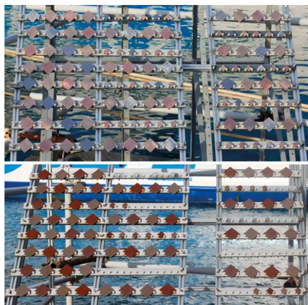
Figure 1. Exposure rack at the beginning (top) and after 14 months exposure (bottom)
