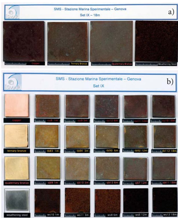
Figure 2. Typical coupons appearance after weathering: a) large samples after 18 months; b) small samples at different exposure times
