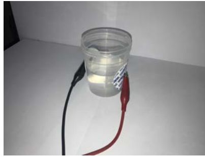
Figure 11: Picture of the level sensor used to determine the level of liquid in the reservoir. If there is not enough culture media the peristaltic pump of the replacement media will be activated to inject some extra fluid. The picture shows a recipient (it is not the final reservoir) with the electrodes and the connections to the electric circuit (the circuit is not included).
