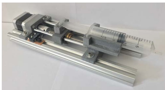
Figure 7: Picture of one of the syringe pumps already built.
