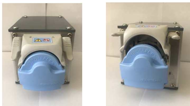
Figure 9: Pictures of the peristaltic pumps for the hemofiltration system and the replacement media.
