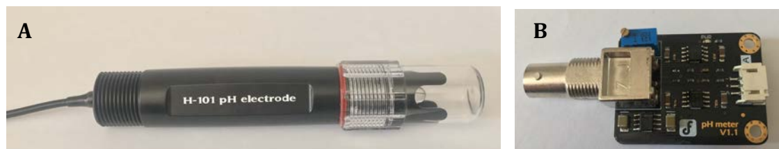
Figure 16: Picture of the pH-meter. (A) The probe. (B) The driver. It is used to control the pH at the reservoir. Its measurements determine the injection of acid or basic solution with the corresponding syringe pumps.
