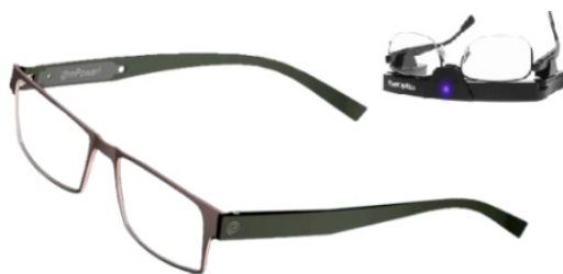
Figure 6. Commercial LC glasses with tunable focus (PixelOptics) [136].
