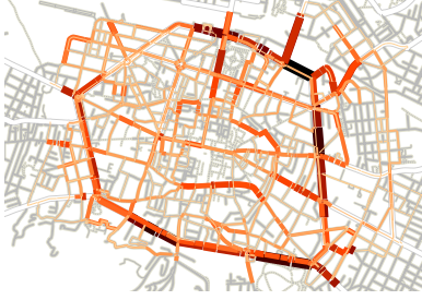
Fig. 1. Bologna Ringway scenario. Road layout, darker colors denote more trafficked road segments.
