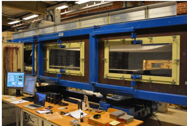
Figure 3.2: Picture from the experimental campaign carried out in the MTL wind tunnel. Panoramic view from the flat plate with a roof geometry.
