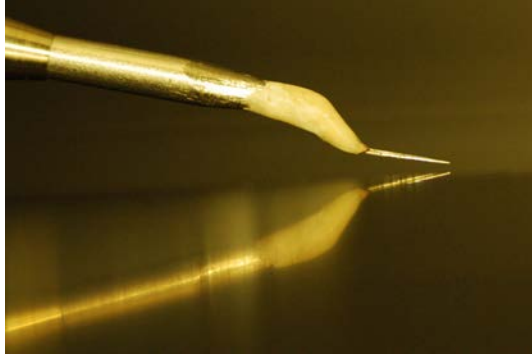
Figure 3.3: Homemade hot-wire probe inside the MTL wind tunnel.
