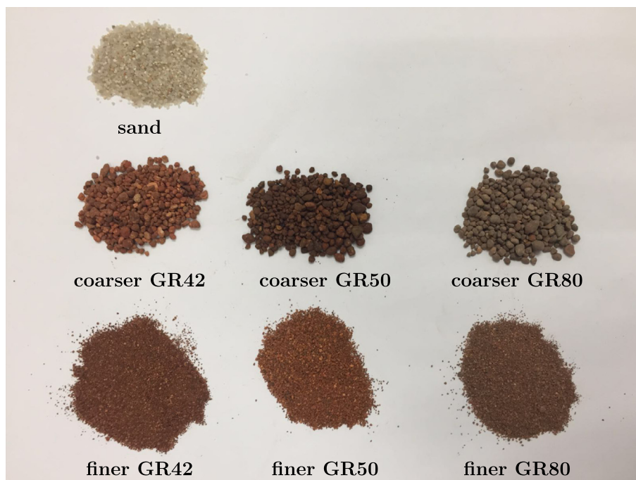
Fig. 1. Images of different granular PCMs that are used for sensible heat storage, and silica sand is also shown as a reference.
