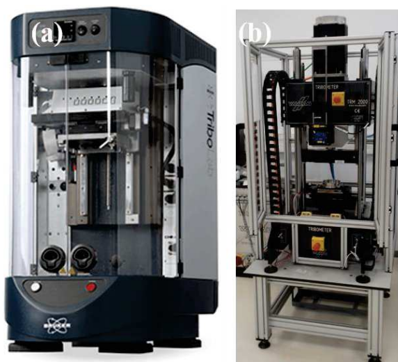
Figure 3.9. Image of sliding wear test equipments: (a) Bruker-UMT-Tribolab and (b) Wazau-TRM 2000-Tribometer.
