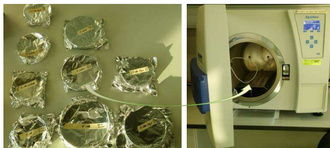
Figure 3.12 Autoclave equipment for sterilization of samples prior to the cell culture studies.
