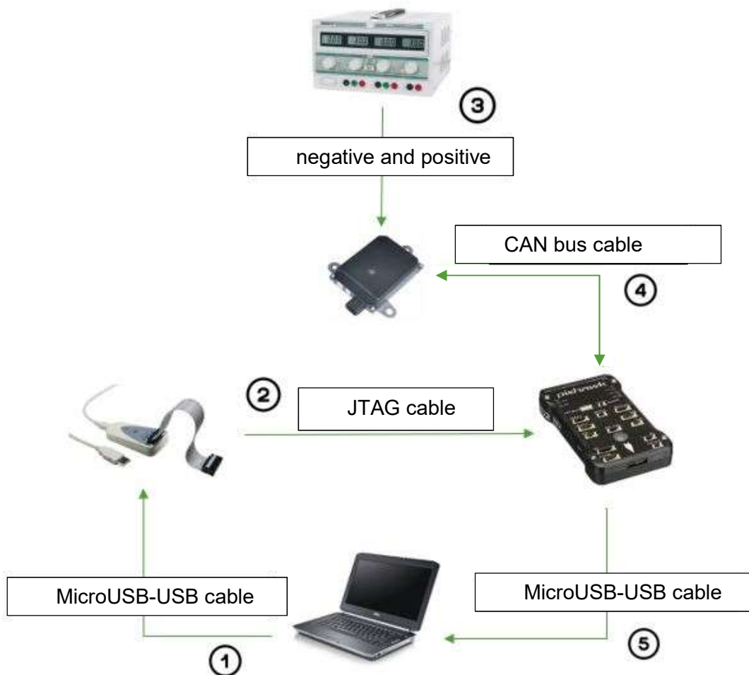
Ilustración 71. Schema of project connections and information flow [30] [31]
