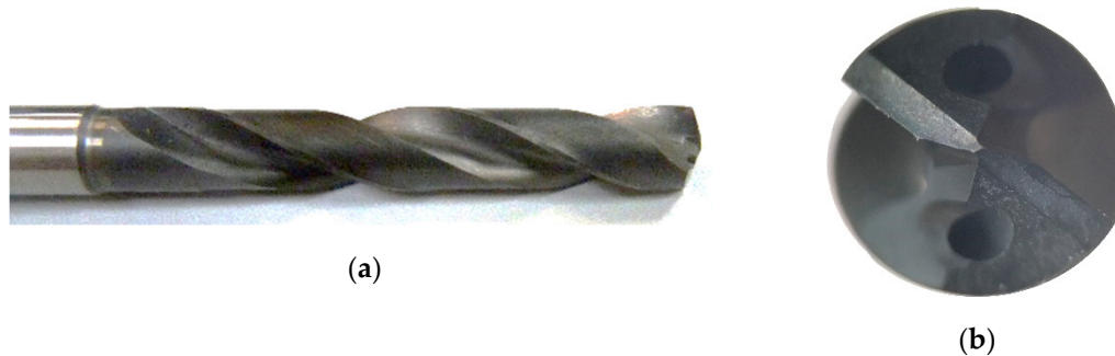
Figure 1. The diamond-coated carbide drill bit with a 7.6 mm diameter that were tested. (a) Lateral view. (b) Frontal view.
