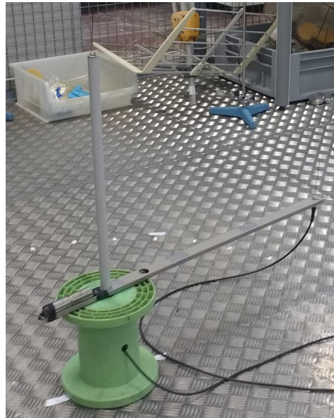
Figure 12. Antenna layout for three dimensional localization.
