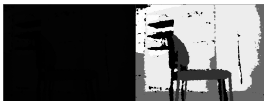
Figure 3. Image obtained from the kinect(left hand side) compared with equalized image (right hand side).
