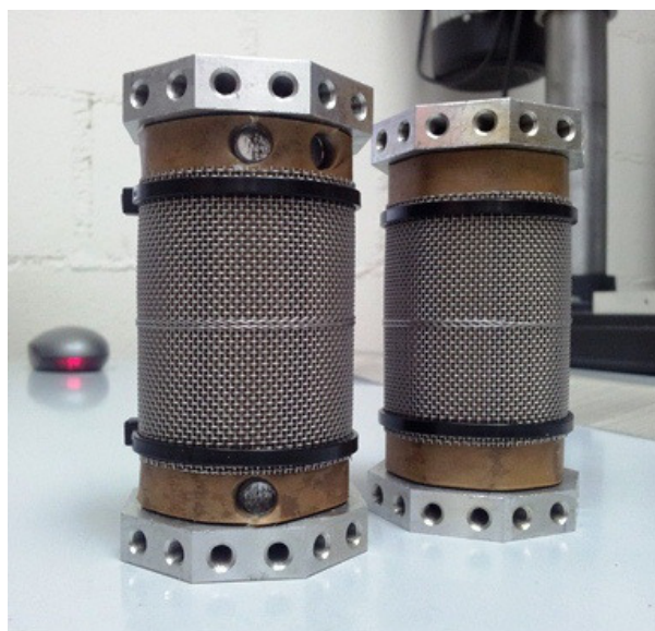
Figure 2. Two prototypes with impregnated paper and metallic mesh belts. The left specimen has three holes where samples have been taken to be analyzed with the Karl Fischer method.
