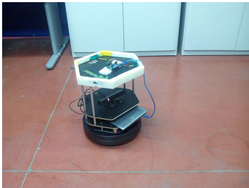
Figure 10. Turtlebot equipped with microphones and Asus 3D-sensor.
