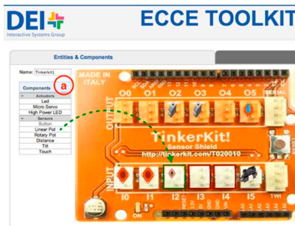
Figure 3. A screenshot of the web interface for the definition of Tinkerkit-based interactive entities. Users can (a) drag-and-drop sensors and actuators from a palette of components to the desired port.
