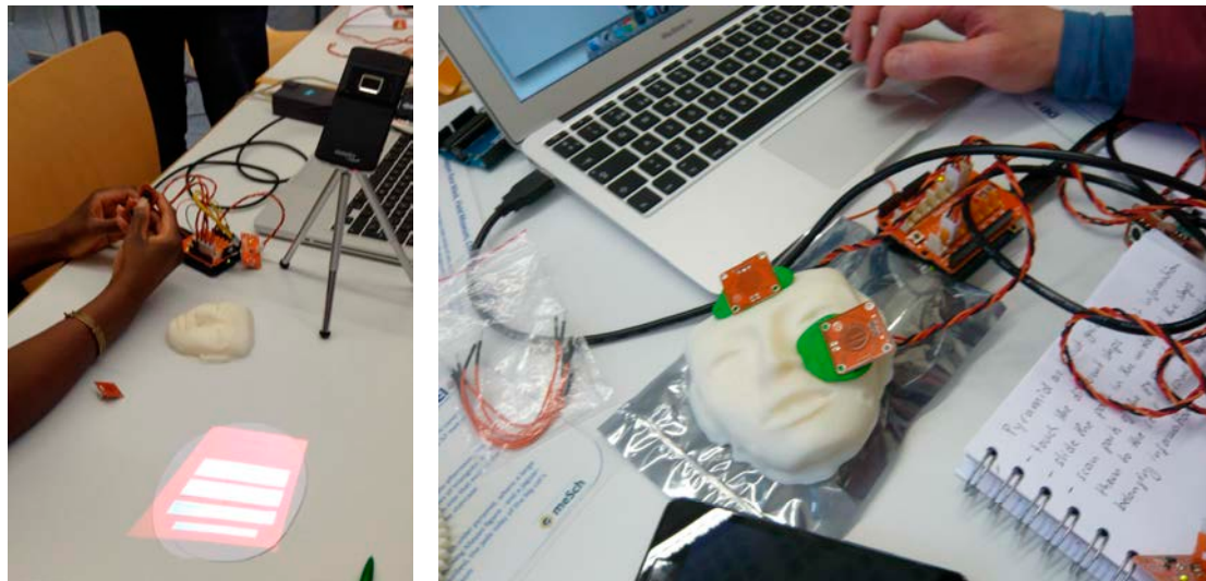
Figure 12. Physical buttons (left) and touch sensors (right) are used to interact with a 3D replica of a funerary mask.
