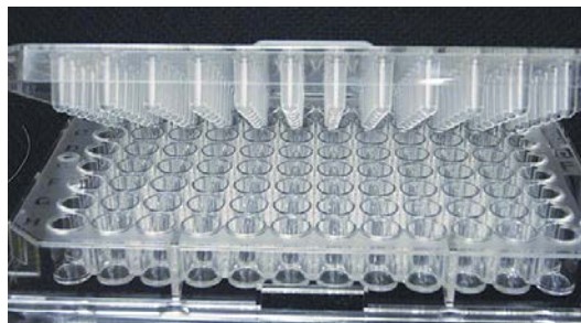
Figure 3. 11 Picture of the polymeric device employed (Calgary device) to treat the mature biofilm and the MC3T3-E1 cells
