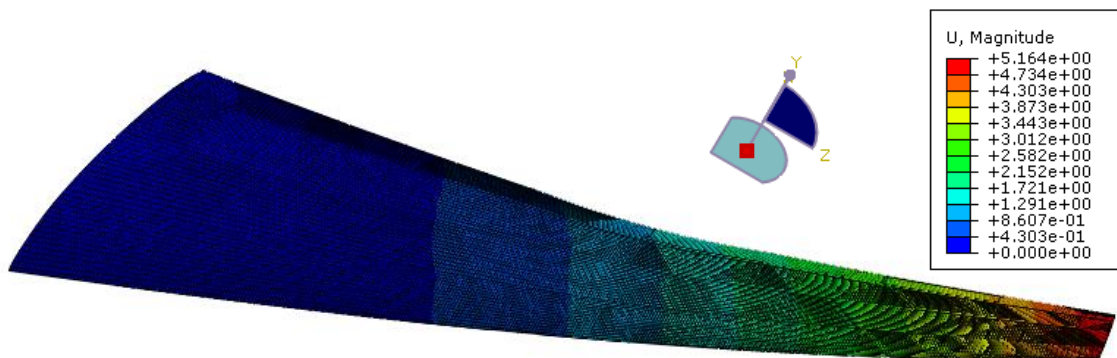
Figure 4.21 - Displacements during Landing
