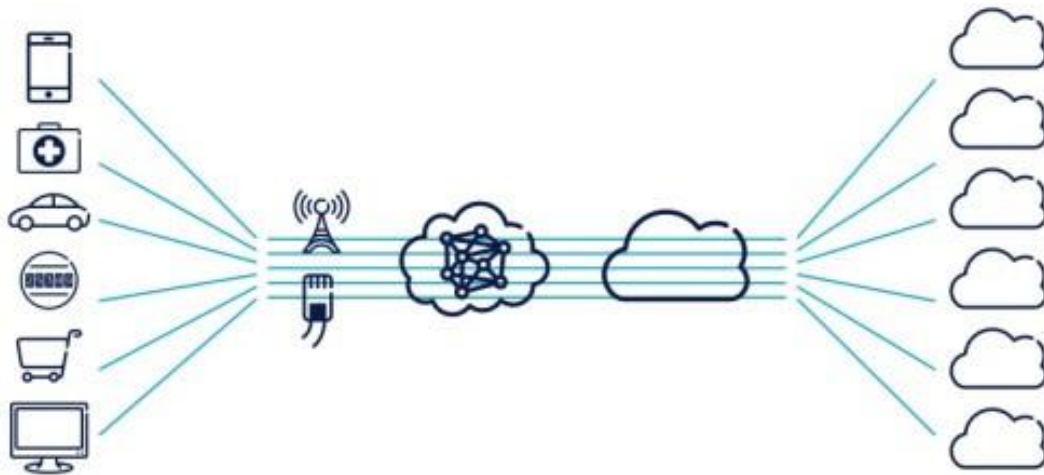
Figure 22. Network slicing diagram. Source: Ericsson via Inside5G [22]
