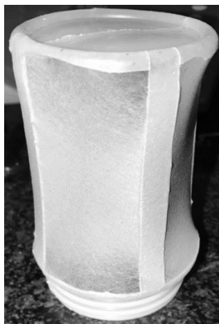
Figure 17. Polymer mat created by undergoing SBS at the before mentioned working conditions.
