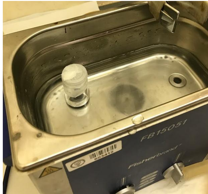
Figure 18. EVA/Cu mixture vial undergoing an ultrasonic bath for 30 minutes.
