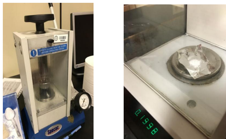
Figure 20. On the left shows the pneumatic press with the lever on his right side. The right picture shows the placement in the electronic balance of KBr.
