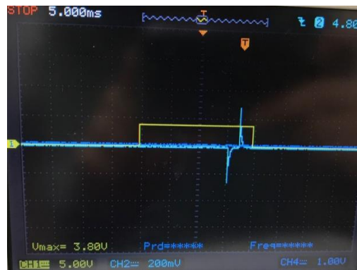
Figure 23: CH1 (yellow): Output A, CH2 (blue): Gate monitor
