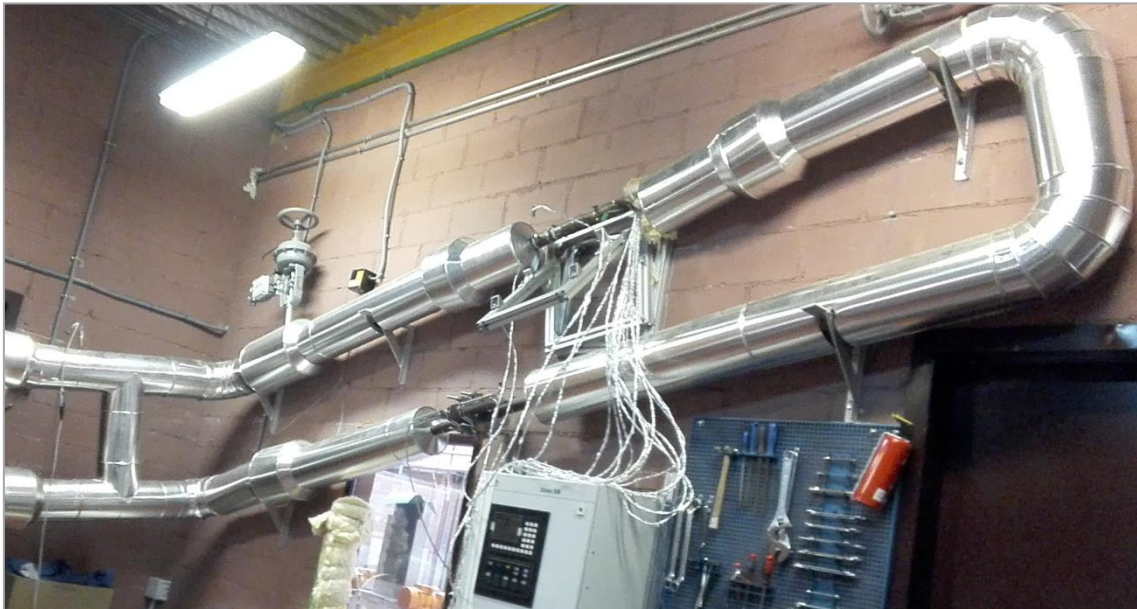
Figure 21: Circulation loop with the non-isolated sections pointed.
