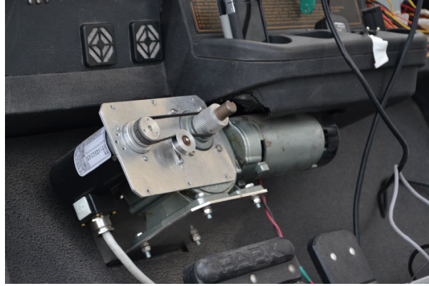
Figure 4.2: Motor-encoder system on iCab1
