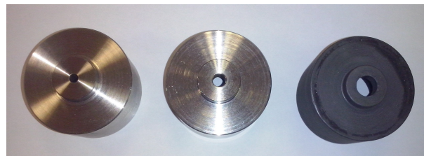
Figure 4.15: Comparison of nozzle throat diameters. From left to right: 4mm, 6mm and 9.5mm
