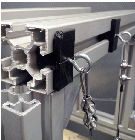
Figure 4.22: Hooks, steel cables and aluminum profile arrangement
