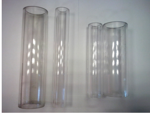
Figure 4.8: Sets of propellant tubes: 210mm on the left and 150mm on the right
