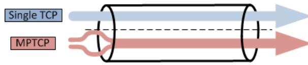
Figure 2.4: A multipath connection should not take up capacity from a coexisting single path connection.
