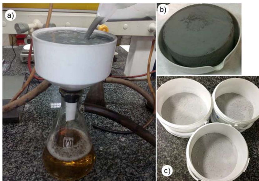
Figure 2.4 a) Separation of the zeolites and mother liquor by filtration. b) Wet zeolite sample. c) Dry zeolite samples.
