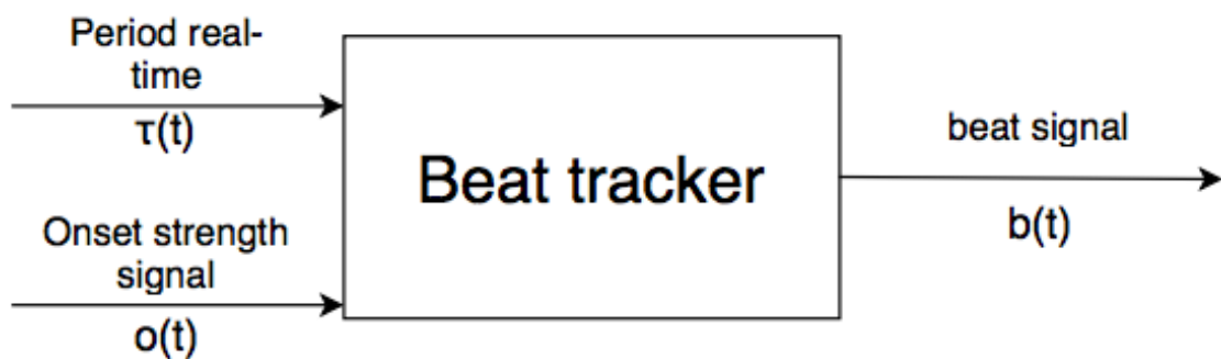
Figure 18: The beat tracker as an input-output system.
