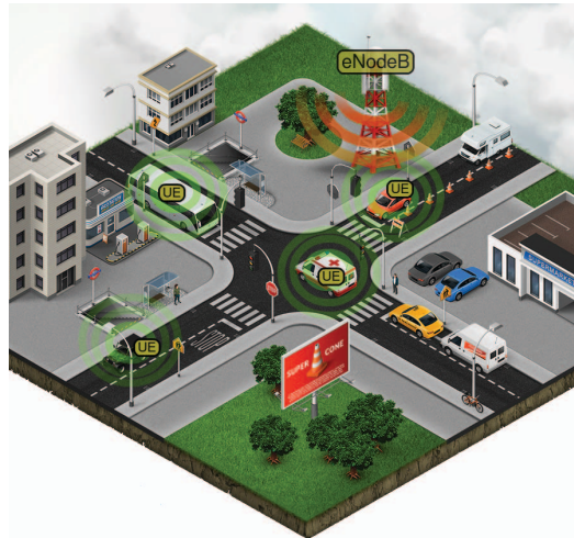
Fig. 1. Simulated scenario, in the version where the LTE technology is used and RSUs are eNodeBs.
