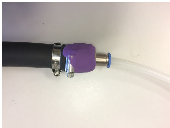
(c) Hose plug-in adapter covered with molding clay.
