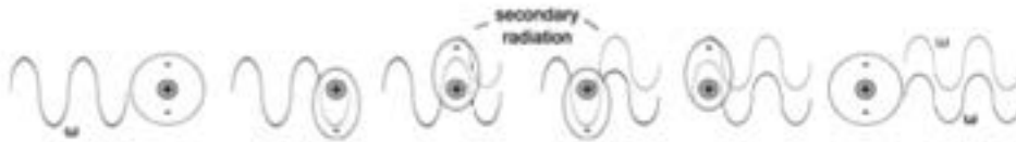
Fig. 6: Schematic of an electromagnetic wave interacting with matter through the Lorentz model. Re-radiation of the incident energy. Figure extracted from [12]
