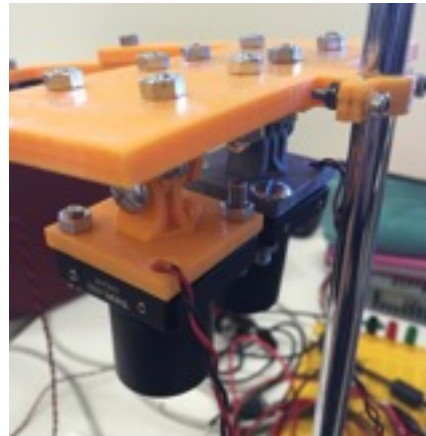
Fig. 12 Pictures of the prototype's base for mounting the LEDs., different views.
